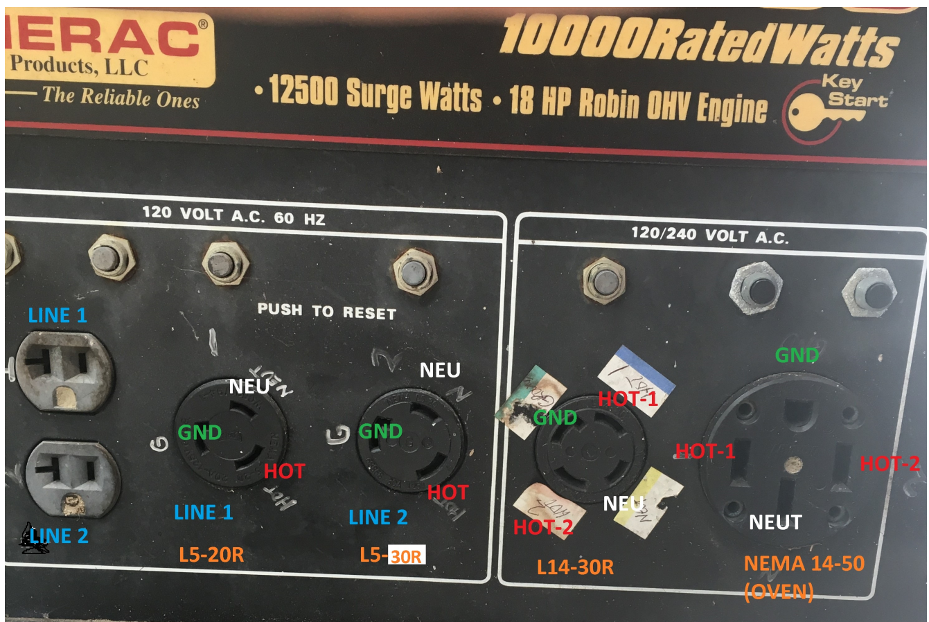
10KW Generator with arbitrary line numbering.
