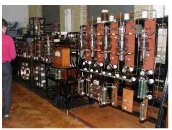
This is 2LO The BBC first transmitter consisting of a 100 watt transmitter.
